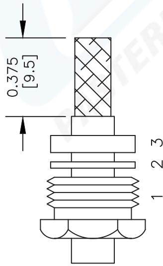
2. FORM BRAID OVER CLAMP NUT (4). TRIM BRAID BACK TO SHOULDER. CUT DIELECTRIC & CENTER CONDUCTOR TO DIMENSION SHOWN. DO NOT NICK CENTER CONDUCTOR. SOLDER CONTACT TO CENTER CONDUCTOR. REMOVE EXCESS SOLDER. DO NOT OVER HEAT DIELECTRIC. INSERT CABLE ASSEMBLY INTO BODY & TIGHTEN.
