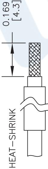
2. AFTER PRE TINNING, TRIM TO DIMENSION SHOWN TO EXPOSE THE CENTER CONDUCTOR
