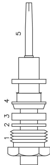
5. REMOVE EXCESS SOLDER. INSERT ASSEMBLY INTO CONNECTOR BODY AND TIGHTEN NUT.
