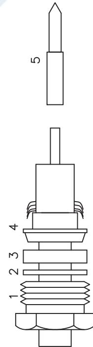
4. INSTALL CONTACT BY SOLDERING TO CABLE CENTER CONDUCTOR LEAVING NO GAPS (5).
