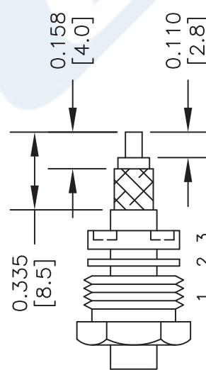
3. a) SLIDE BRAID CLAMP OVER BRAID UNTIL IT STOPS ON CABLE JACKET.
