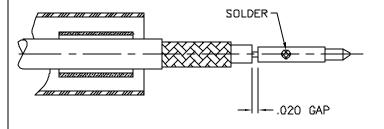
2) A. Slide contact onto center conductor leaving a .020 gap as shown and solder to center conductor. Use minimal heat to minimize melting of foam dielectric. Inspect to be sure aluminum foil is not touching center contact.
