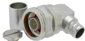
N Male Right Angle Connector Crimp/Solder Attachment for PE-C400, PE-B400, PE-B405, LMR-400, LMR-400-DB, LMR-400-UF, 0.400 inch
