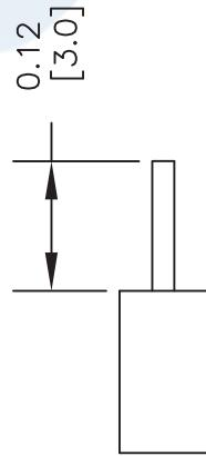
2. INSERT BODY THROUGH CABLE. PLACE WASHER OVER CENTER CONDUCTOR. PLACE CONTACT OVER CONDUCTOR UNTIL IT BOTTOMS OUT. SOLDER CONTACT TO CENTER CONDUCTOR AS SHOWN.
