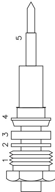
5. REMOVE EXCESS SOLDER. INSERT ASSEMBLY INTO CONNECTOR BODY AND TIGHTEN NUT.
