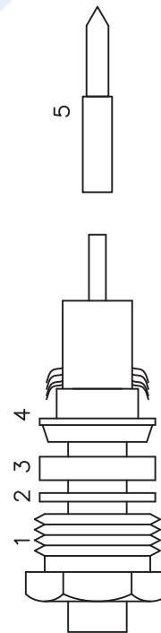
4. INSTALL CONTACT BY SOLDERING TO CABLE CENTER CONDUCTOR LEAVING NO GAPS (5).
