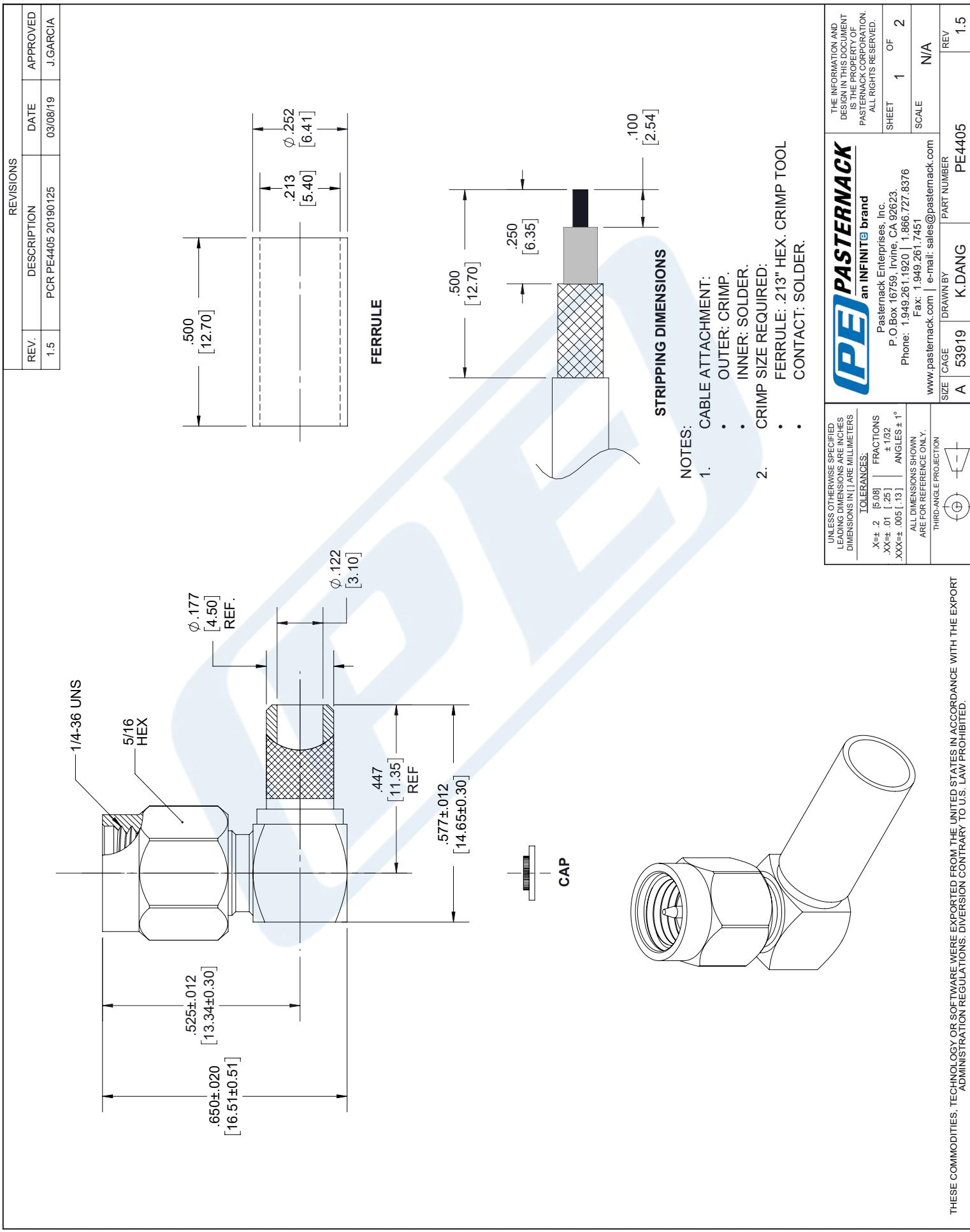
TNC Male Connector Crimp/Solder Attachment for RG58,
