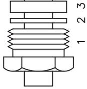
2. FORM BRAID OVER CLAMP NUT (4). TRIM BRAID BACK TO SHOULDER. CUT DIELECTRIC & CENTER CONDUCTOR TO DIMENSION SHOWN. DO NOT NICK CENTER CONDUCTOR. SOLDER CONTACT TO CENTER CONDUCTOR. REMOVE EXCESS SOLDER. DO NOT OVER HEAT DIELECTRIC. INSERT CABLE ASSEMBLY INTO BODY & TIGHTEN.
