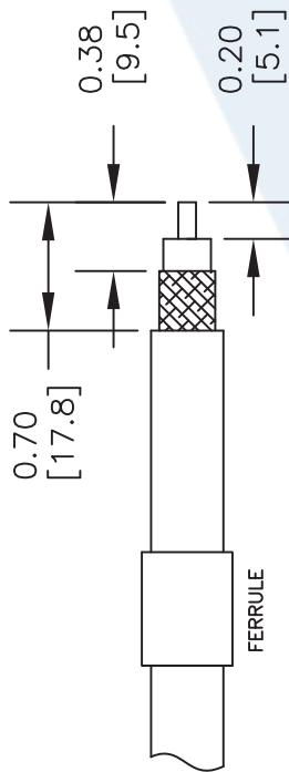
2. FLAIR BRAID AND INSERT THE STRIPPED CABLE INTO BODY AND POSITION THE CENTER CONDUCTOR IN THE SLOT OF THE CENTER PIN.
