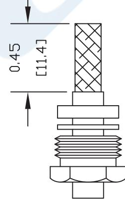
2. FORM BRAID OVER CLAMP NUT (4). CUT DIELECTRIC TO DIMENSION SHOWN. DO NOT NICK CENTER CONDUCTOR. TIN CENTER CONDUCTOR. SLIDE ASSEMBLY INTO BODY, SOLDER CENTER CONDUCTOR IN PLACE & TIGHTEN CLAMP NUT. SCREW CAP DOWN INTO PLACE.
