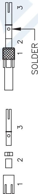
3. CLEAN EXCESS SOLDER. SLIDE ASSEMBLY INTO BODY. SLIDE FERRULE (1) INTO BODY. ALLOW .05" CRIMP SPACE BEFORE BODY (4).
