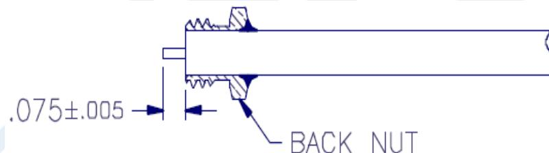
2. SLIDE BACK NUT ONTO CABLE UNTIL TRIMMED END OF JACKET IS FLUSH WITH FRONT OF NUT. SOLDER NUT TO CABLE.
