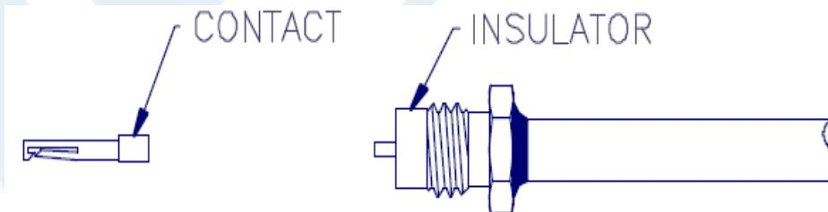
4. INSTALL INSULATOR OVER CABLE CENTER CONDUCTOR.
