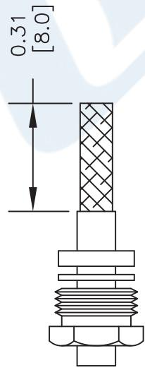
2. FORM BRAID OVER CLAMP NUT (4). TRIM BRAID BACK TO SHOULDER. CUT DIELECTRIC & CENTER CONDUCTOR TO DIMENSION SHOWN. DO NOT NICK CENTER CONDUCTOR. SOLDER CONTACT TO CENTER CONDUCTOR. REMOVE EXCESS SOLDER. DO NOT OVER HEAT DIELECTRIC. INSERT CABLE ASSEMBLY INTO BODY & TIGHTEN.
