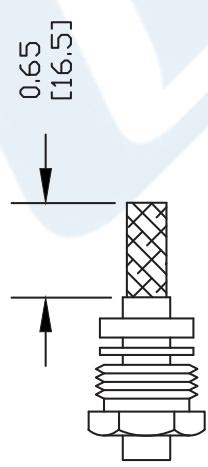
2. FORM BRAID OVER CLAMP NUT (4). TRIM BRAID BACK TO SHOULDER. CUT DIELECTRIC & CENTER CONDUCTOR TO DIMENSION SHOWN. DO NOT NICK CENTER CONDUCTOR. TIN CENTER CONDUCTOR SLIDE ASSEMBLY INTO BODY, SOLDER CENTER CONDUCTOR IN PLACE, TIGHTEN CLAMP NUT & SCREW CAP
