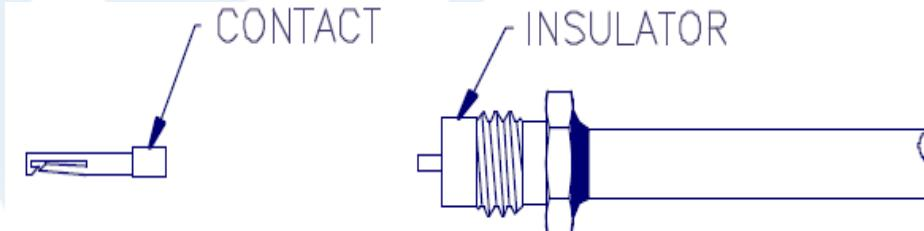
4. INSTALL INSULATOR OVER CABLE CENTER CONDUCTOR.
