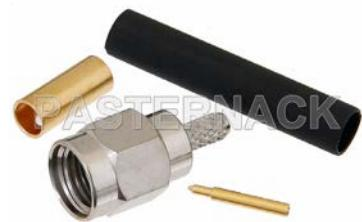
SMA Male Connector Solder Attachment for RG174, RG316, RG188, LMR-100, PE-B100, PE-C100, 0.100 inch
