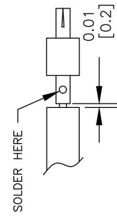
3. INSERT CABLE FULLY INTO BODY. SOLDER OUTER CONDUCTOR TO BODY.
