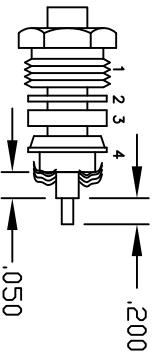
NOTE: INSERT PTFE BEFORE CONTACT WITH LARGE OPEN END SLIDING OVER CENTER CONDUCTOR & DIELECTRIC.
