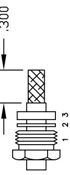
2. FORM BRAID OVER CLAMP NUT (4). TRIM BRAID BACK TO SHOULDER. CUT DIELECTRIC & CENTER CONDUCTOR TO DIMENSION SHOWN. DO NOT NICK CENTER CONDUCTOR. SOLDER CONTACT TO CENTER CONDUCTOR. REMOVE EXCESS SOLDER. DO NOT OVER HEAT DIELECTRIC. INSERT CABLE ASSEMBLY INTO BODY & TIGHTEN.
