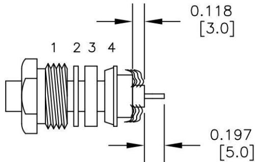
Click the following link (or enter part number in "SEARCH" on website) to obtain additional part information including price, inventory and certifications: [N Male Connector Clamp/Solder Attachment for RG213, RG214, RG8, RG9, RG11, RG225, RG393, RG144, RG216, RG215 PE4062](#)
