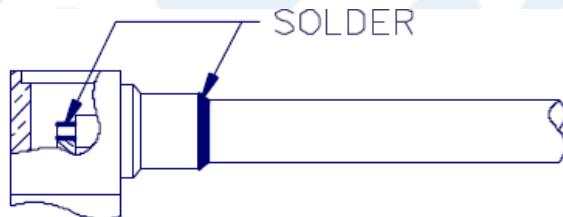
3. SOLDER CENTER CONDUCTOR TO CONTACT.
