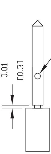
3. SLIDE INSULATOR OVER CONTACT UNTIL IT BOTTOMS OUT. INSERT INSULATOR TO BODY UNTIL IT MATES. SOLDER BODY TO CABLE.
