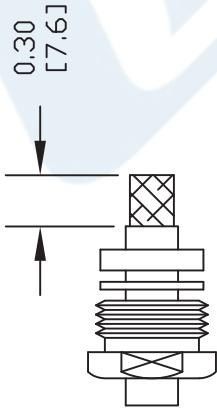
2. FORM BRAID OVER CLAMP NUT (4). TRIM BRAID BACK TO SHOULDER. CUT DIELECTRIC & CENTER CONDUCTOR TO DIMENSION SHOWN. DO NOT NICK CENTER CONDUCTOR. SOLDER CONTACT TO CENTER CONDUCTOR. REMOVE EXCESS SOLDER. DO NOT OVER HEAT DIELECTRIC. INSERT CABLE ASSEMBLY INTO BODY & TIGHTEN.
