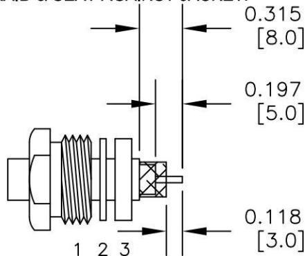
2. FORM BRAID OVER CLAMP NUT (4). CUT DIELECTRIC AND CENTER CONDUCTOR TO DIMENSION SHOWN. DO NOT NICK CENTER CONDUCTOR. SOLDER CONTACT TO CENTER CONDUCTOR. REMOVE EXCESS SOLDER. DO NOT OVER HEAT DIELECTRIC. INSERT CABLE ASSEMBLY INTO BODY & TIGHTEN.
