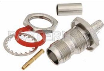
TNC Female Bulkhead Mount Connector Crimp/Solder Attachment for RG58, RG303, RG141, PE-C195, PE-P195, LMR-195, 0.195 inch, .480 inch D Hole
