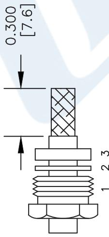
FORM BRAID OVER CLAMP NUT (4). TRIM BRAID BACK TO SHOULDER. CUT DIELECTRIC & CENTER CONDUCTOR TO DIMENSION SHOWN. DO NOT NICK CENTER CONDUCTOR. SOLDER CONTACT TO CENTER CONDUCTOR. REMOVE EXCESS SOLDER. DO NOT OVER HEAT DIELECTRIC. INSERT CABLE ASSEMBLY INTO BODY & TIGHTEN.
