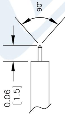
2. SOLDER CONTACT TO CENTER CONDUCTOR MAINTAINING INDICATED SPACING.
