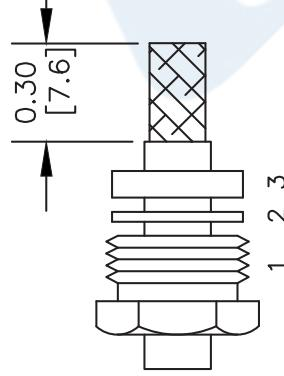
2. FORM BRAID OVER CLAMP NUT (4). TRIM BRAID BACK TO DIMENSION SHOWN. CUT DIELECTRIC & CENTER CONDUCTOR TO DIMENSION SHOWN. DO NOT NICK CENTER CONDUCTOR. SOLDER CONTACT TO CENTER CONDUCTOR. REMOVE EXCESS SOLDER. DO NOT OVER HEAT DIELECTRIC. INSERT CABLE ASSEMBLY INTO BODY & TIGHTEN.
