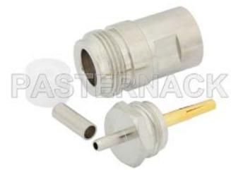
N Female Connector Crimp/Solder Attachment for RG174, RG316, RG188, LMR-100, PE-B100, PE-C100, 0.100 inch
