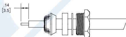
3. SOLDER CONTACT (5) TO CENTER CONDUCTOR. REMOVE EXCESS SOLDER. DO NOT OVER HEAT DIELECTRIC. INSERT CABLE ASSEMBLY INTO BODY (6) & TIGHTEN.
