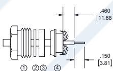
3. SLIDE INSULATOR (5) AGAINST THE BRAID CLAMP. SOLDER CONTACT (6) TO CENTER CONDUCTOR. REMOVE EXCESS SOLDER. DO NOT OVER HEAT DIELECTRIC. INSERT CABLE ASSEMBLY INTO BODY (7) & TIGHTEN WITH RECOMMENDED TORQUE: 16 in-lbs.
