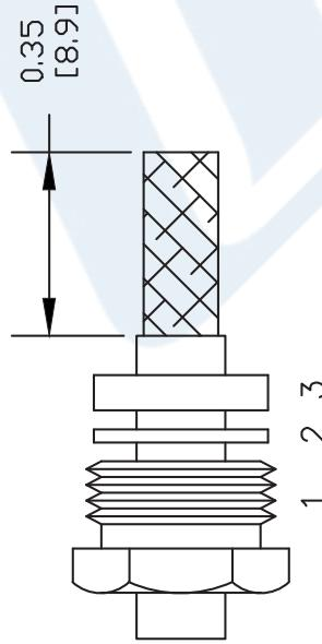
2. FORM BRAID OVER CLAMP NUT (4). TRIM BRAID BACK TO SHOULDER. CUT DIELECTRIC & CENTER CONDUCTOR TO DIMENSION SHOWN. DO NOT NICK CENTER CONDUCTOR. SOLDER CONTACT TO CENTER CONDUCTOR. REMOVE EXCESS SOLDER. DO NOT OVER HEAT DIELECTRIC. INSERT CABLE ASSEMBLY INTO BODY & TIGHTEN.
