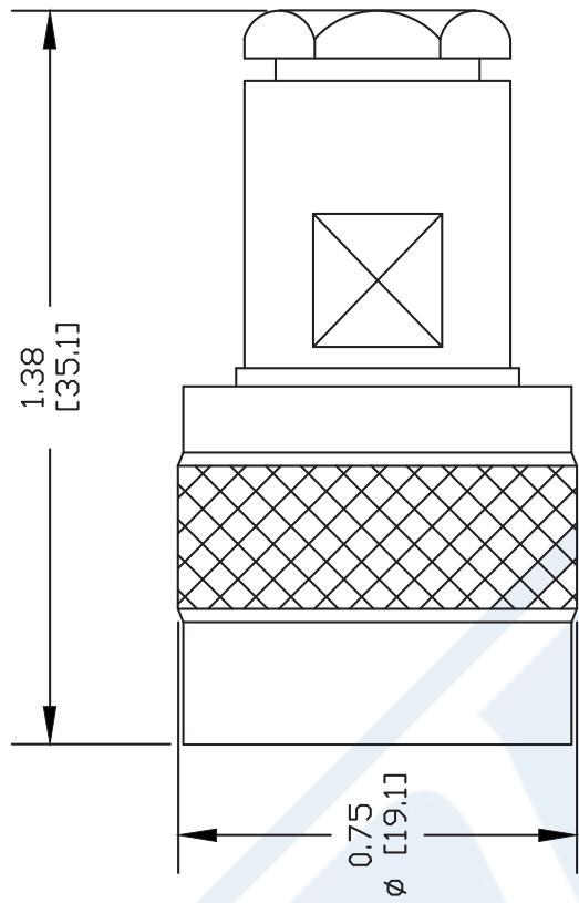
2. FORM BRAID OVER CLAMP NUT (4). TRIM BRAID BACK TO SHOULDER. CUT DIELECTRIC & CENTER CONDUCTOR TO DIMENSION SHOWN. DO NOT NICK CENTER CONDUCTOR. SOLDER CONTACT TO CENTER CONDUCTOR. REMOVE EXCESS SOLDER. DO NOT OVER HEAT DIELECTRIC. INSERT CABLE ASSEMBLY INTO BODY & TIGHTEN.
