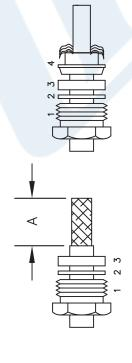
CONTACTS. LINE THE KEY WAY UP WITH THE PIN IN THE STRIP CABLE AS SHOWN IN B. SLIDE BUSHING (5) OVER CONTACTS TO CENTER CONDUCTORS, REMOVE ANY EXCESS SOLDER. PUSH OUT INSULATOR FROM BODY. DIELECTRIC & SEAT FIRMLY AGAINST BRAID. SOLDER BODY & INSERT THE ENTIRE ASSEMBLY INTO BODY & SPREAD OUT CONTACTS. SLIDE INSULATOR OVER LIGHTEN ς.
