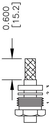
2. FORM BRAID OVER CLAMP NUT (4). CUT DIELECTRIC TO DIMENSION SHOWN. DO NOT NICK CENTER CONDUCTOR. TIN CENTER CONDUCTOR. SLIDE ASSEMBLY INTO BODY, SOLDER CENTER CONDUCTOR, TIGHTEN CLAMP NUT & SCREW CAP IN PLACE.
