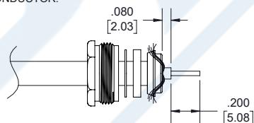
3. SLIDE THICK-WASHER ⑤ AND HALF- INSULATOR ⑥ AGAINST THE BRAID CLAMP AND HOLD BRAID IN PLACE. SOLDER CONTACT ⑦ TO CENTER CONDUCTOR. REMOVE EXCESS SOLDER. DO NOT OVER HEAT DIELECTRIC. SLIDE A REST HALF- INSULATOR ⑥ TO LOCKED CONTACT. INSERT CABLE ASSEMBLY INTO BODY ⑧ & TIGHTEN.
