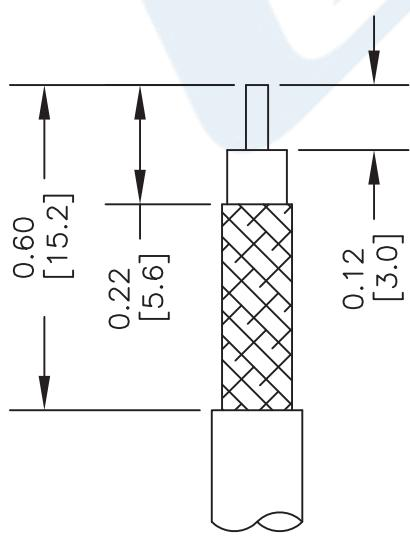
STRIPPING DIMENSIONSASSEMBLY PROCEDURES
