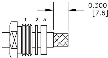
2. FORM BRAID OVER CLAMP NUT (4). TRIM BRAID BACK TO SHOULDER. CUT DIELECTRIC & CENTER CONDUCTOR TO DIMENSION SHOWN. DO NOT NICK CENTER CONDUCTOR. SOLDER CONTACT TO CENTER CONDUCTOR. REMOVE EXCESS SOLDER. DO NOT OVER HEAT DIELECTRIC. INSERT CABLE ASSEMBLY INTO BODY & TIGHTEN.
