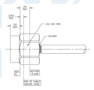
Click the following link (or enter part number in "SEARCH" on website) to obtain additional part information including price, inventory and certifications: SMA Male Connector Solder Attachment for RG405, RG405 Tinned, PE-SR405AL, PE-SR405FL, PE-SR405TN PE45480
