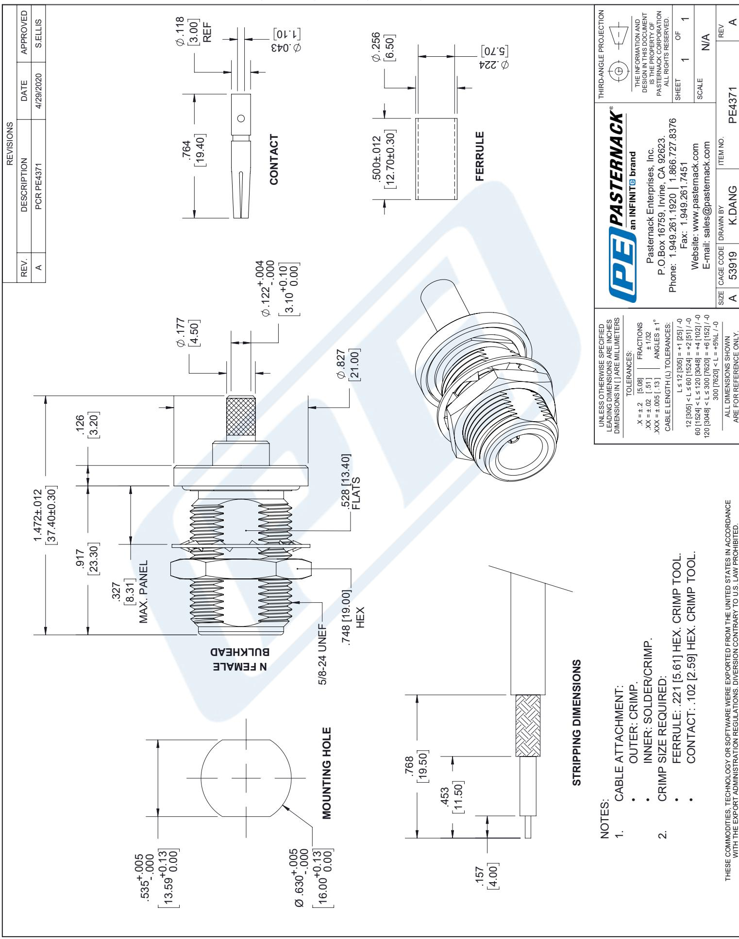
N Female Connector Clamp/Solder Attachment for
