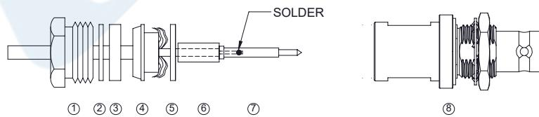
Click the following link (or enter part number in "SEARCH" on website) to obtain additional part information including price, inventory and certifications: [SHV Jack Bulkhead Mount Connector Clamp/Solder Attachment for RG174, RG316, RG188, .480 inch D Hole PE45556](#)
