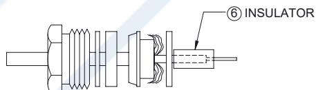
3. SLIDE THICKER WASHER ⑤ AND INSULATOR ⑥ AGAINST THE BRAID CLAMP. SOFT SOLDER CONTACT ⑦ TO CENTER CONDUCTOR. REMOVE EXCESS SOLDER. DO NOT OVER HEAT DIELECTRIC. INSERT CABLE ASSEMBLY INTO BODY ⑧ & TIGHTEN BY CLAMP NUT ONLY.
