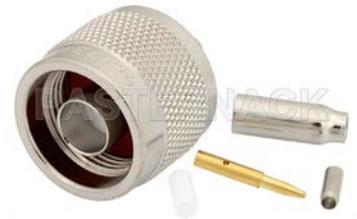
N Male Connector Crimp/Solder Attachment for RG174, RG316, RG188, LMR-100, PE-B100, PE-C100, 0.100 inch
