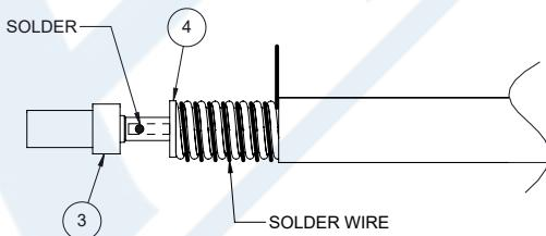
3. PUSH THE CONNECTOR BODY INTO THE CABLE, UNTIL IT STOPS. SOLDER THE CONNECTOR BODY WITH CABLE AND COVER HEATSHRINK SLEEVE.
