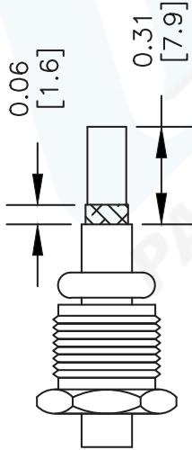
2. FLARE BRAID, SLIDE CLAMP OVER AND UNDER BRAID UNTIL THE CLAMP STOPS. TRIM EXCESS BRAID TO THE DIAMETER OF CLAMP SHOULDER. TRIM CABLE TO DIMENSIONS SHOWN. DO NOT NICK CENTER CONDUCTOR.
