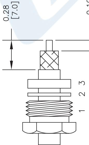
2. FORM BRAID OVER CLAMP NUT (4). SOLDER CONTACT TO CENTER CONDUCTOR. REMOVE EXCESS SOLDER. DO NOT OVER HEAT DIELECTRIC. INSERT CABLE ASSEMBLY INTO BODY & TIGHTEN.
