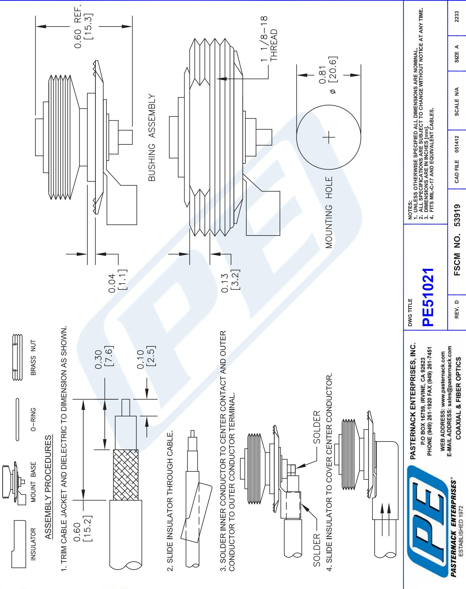
N Female Connector Clamp/Solder Attachment for
