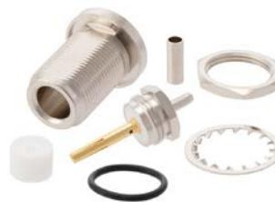
N Female Bulkhead Mount Connector Crimp/Solder Attachment for RG174, RG316, RG188, LMR-100, PE-B100, PE-C100, 0.100 inch, .640 inch DD Hole
