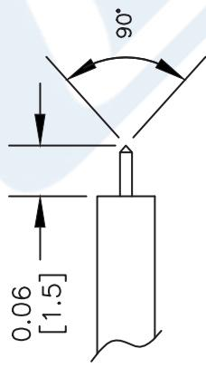
2. SOLDER CONTACT TO CENTER CONDUCTOR MAINTAINING INDICATED SPACING.
